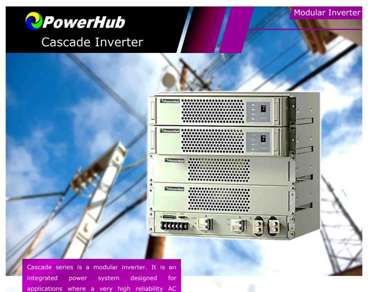
These compact parallel inverter module can be configured to meet the N+X requirements. While the modules are in the type of rackmout, all of them can be hot-swapped without disturbing the AC load. Each module is 3KVA and system is able to cascade up to 4 modules in parallel.
